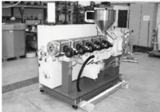
**HELIBAR®** technology (grooved barrel and barrier-screw) has been developed and patented by EXTRUDEX.
