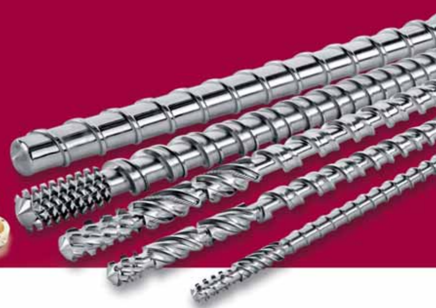
Screws and barrels • Screws and barrels available in standard and custom designs for processing of thermoplastic resins. • Broad spectrum of screw types and designs available in diameters from 12 mm to over 150 mm and lengths up to 4500 mm. • Advanced coatings with hardness up to the range 68-71 HRC (Rockwell "C" hardness) permit processing of even difficult-to-plastify resins.
